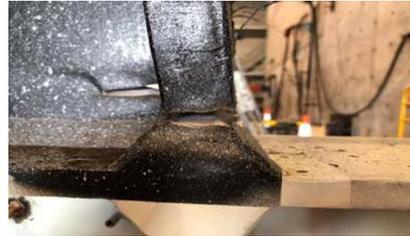
Figure 7. Specimen 3 after failure.
