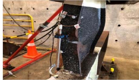
Figure 6. Specimen 2 after failure.
